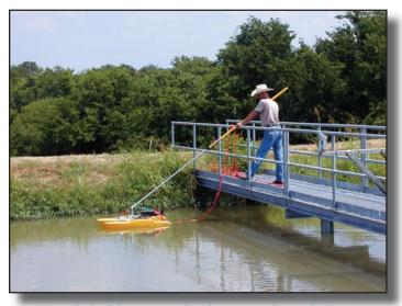
David Murdoch of the Lower Colorado River Authority deploys a trimaran-mounted RiverSurveyor to measure flow throughout the vertical water column. In obstructed reaches, the instrument's stationary software delivers excellent data to a simple, intuitive interface, says Murdoch's colleague, Keith Ging.
