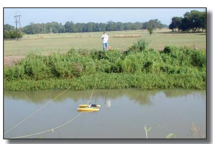
A Lower Colorado River Authority hydrologist remotely directs a catamaran mounted RiverSurveyor along a transect across a canal. Along a transect or using stationary software, the RiverSurveyor uses Doppler sonar to quickly, accurately measure flow in the vertical water column.
